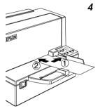
3. After printing is complete, the SLIP LED goes off, and you can remove the slip.
