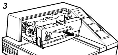
6. Before installing the new ribbon, check that it is not creased or twisted. Then turn the feed knob in the direction of the arrow on the ribbon cassette to take up any slack in the ribbon.
